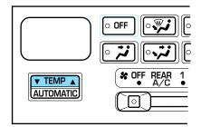
For continuous maximum cooling, push the temperature control until 15°C (60°F) is shown in the display window. The EATC will continue maximum cooling (disregarding the displayed temperature) until a warmer temperature is selected by pressing the temperature controls.
